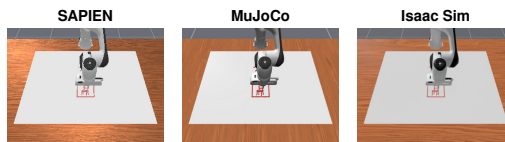
Figure 4: Cross-simulator deployment of the BURGER trajectory-generation pipeline. The same SVG drawing task is executed in SAPIEN, MuJoCo, and Isaac Sim using corresponding robot-control interfaces.
